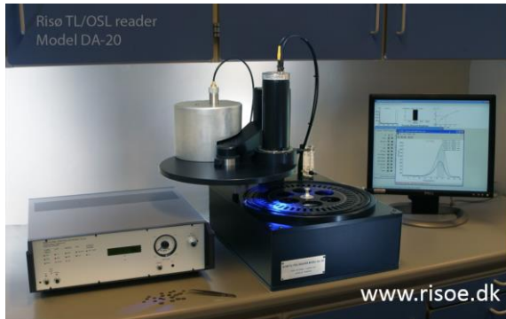
Fig. 3. Riso TL/OSL reader Model DA-20 with a bialkali EMI 9235QA PMT
