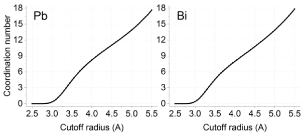
Fig. 2. An alternative way to express correlation functions. In the coordination number – cutoff radius relationship, the derivative of the graph represents the correlation function.
