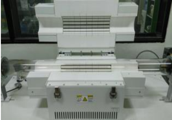
Fig. 2 Severe accident environment simulation equipment for ES evaluation (KIMM-SAES)
