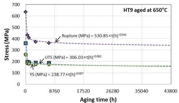
Fig. 4. Mechanical properties change of HT9 as function of aging time [13].
