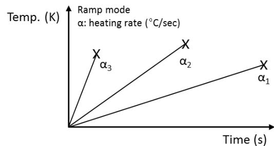
Fig. 1. Typical ramp test mode of transient test.
