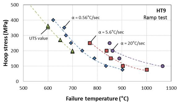
Fig. 2. Result of the ramp tests (with ramp rate of 0.56, 5.6, and 20°C/sec, respectively) compared to the UTS value [14] of HT9.
