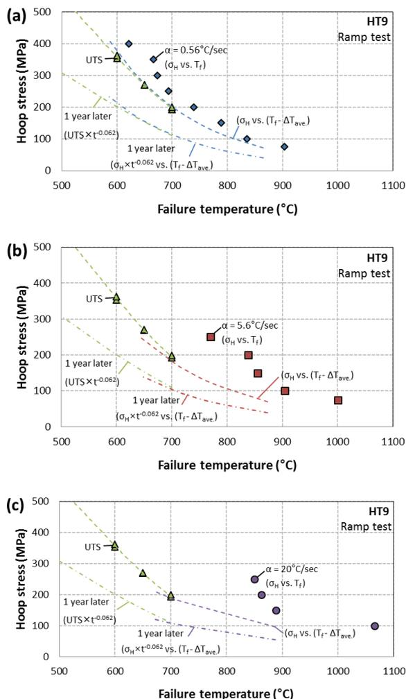
Fig. 5. Aging effect of HT9 cladding tube on transient (ramp test) behavior at (a)  $0.56^\circ\text{C/sec}$ , (b)  $5.6^\circ\text{C/sec}$ , and (c)  $20^\circ\text{C/sec}$ .
