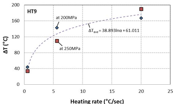
Fig. 3. Temperature difference (between a uniform temperature during the tensile test and a failure temperature of a transient) as function of heating rate.
