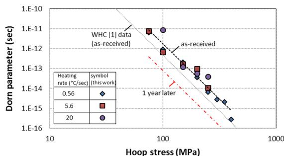
Fig. 6. Dorn parameter from as-received and estimated aging effect with 1 year later as a function of hoop stress.
