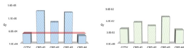
Fig. 4. Gamma-rays (left) and neutrons (right) cumulative dose of the IHVS during 10 years
