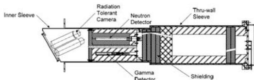
Fig. 1. The schematic of a camera-radiation detector (CRD), composed of a He-3 neutron detector, a gamma detector and two radiation-tolerant cameras, which has been applied in the head-end process of the Rokkasho reprocessing plant in Japan.
