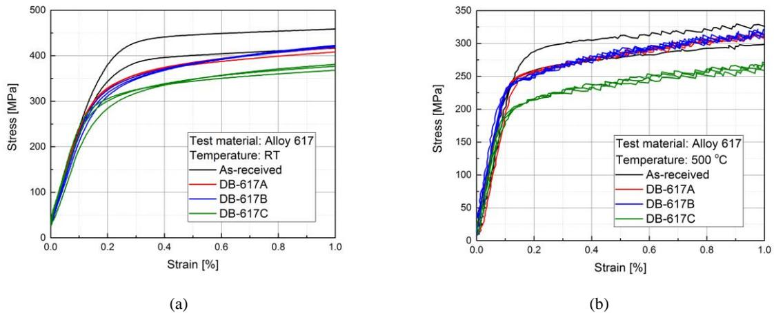
Fig. 1 Stress-strain curves of the as-received and diffusion-welded Alloy 617 up to the strain range of 1 %: (a) room temperature and (b) 500 °C
