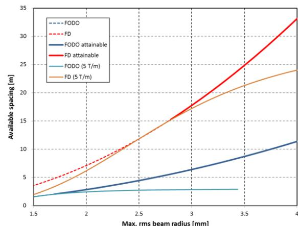
Fig. 2. Distance between magnets depending on beam radius for both FODO and doublet lattice.
