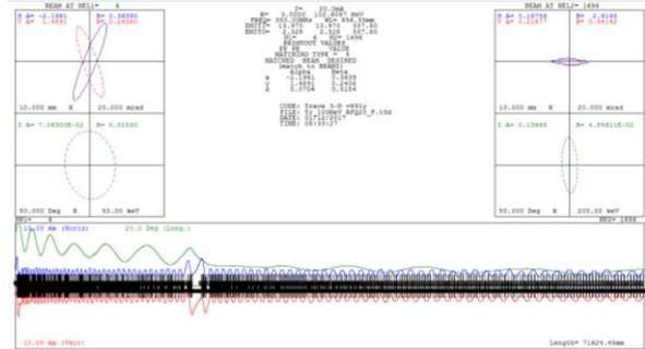
Fig. 1. Beam envelope along the 100-MeV linac.
