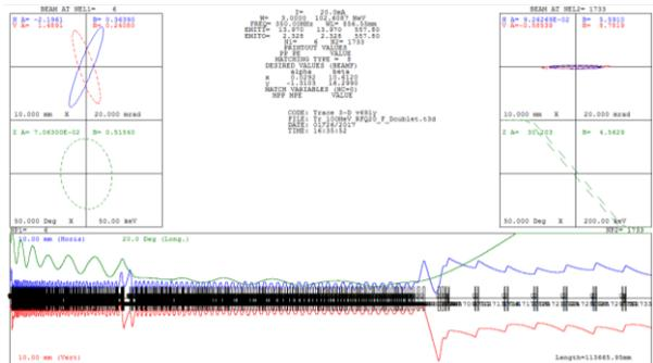
Fig. 4. Beam envelope along the straight beam transport line after 100-MeV accelerator in doublet lattice.
