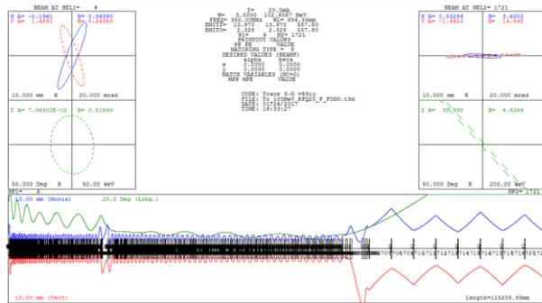
Fig. 3. Beam envelope along the straight beam transport line after 100-MeV accelerator in FODO lattice.
