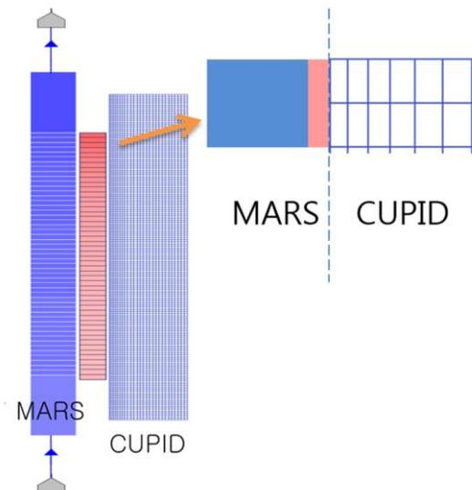
Fig. 2. Schematic diagram of CUPID-MARS coupling calculation
