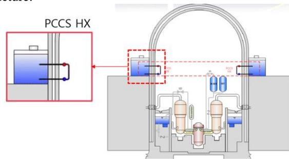
Fig. 1. Schematic diagram of the IPOWER PCCS [5]
