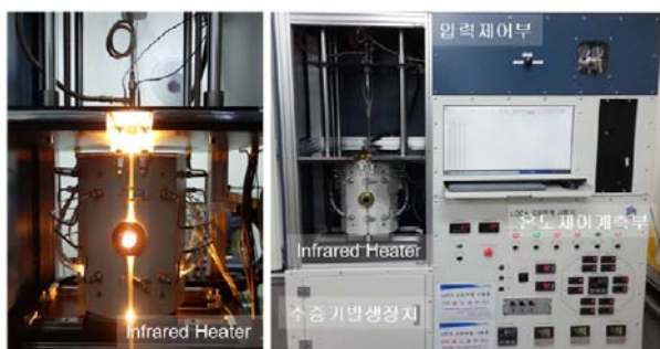
Fig. 1. LOCA burst test system.
