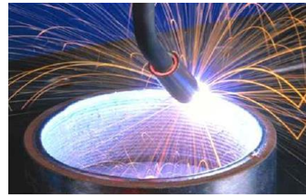
Fig. 2. Overlay-welding process to bond each composite material
