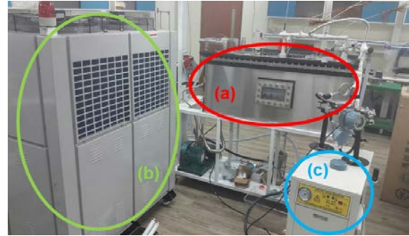
Fig. 3. Photograph of experimental facility ((a): test shell, (b): cooler, (c): steam generator).
