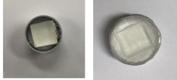
Figure 2. The encapsulated NaI 1 with Teflon sheet (left), encapsulated NaI 2 with MgO powder (right).
