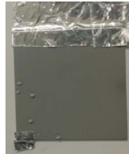
Fig. 4. Attached droplets on the S.A.M coated Al plate.
