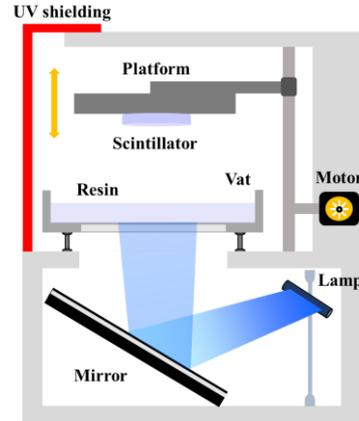
Figure 1. Basic concept of DLP 3D printer.
