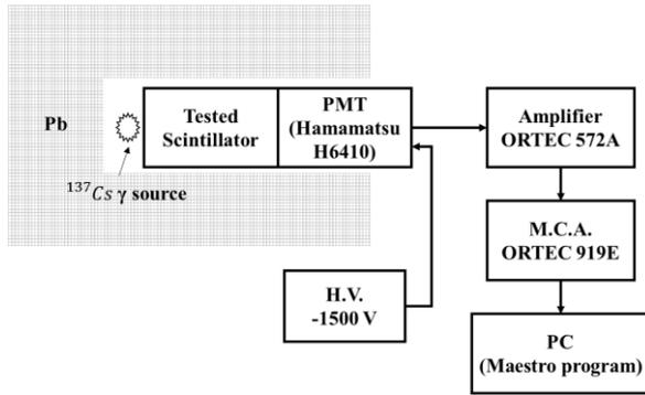
Figure 2. Schematic view of gamma-ray measurement.
