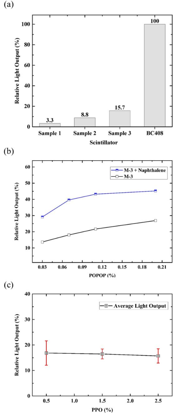
Figure 3. Relative light output (a) with respect to monomers M-1, M-2, M-3 and BC408, (b) POPOP concentrations and addition of naphthalene and (c) PPO concentrations. Relative light output is based on that of the commercial plastic scintillator (BC408).
