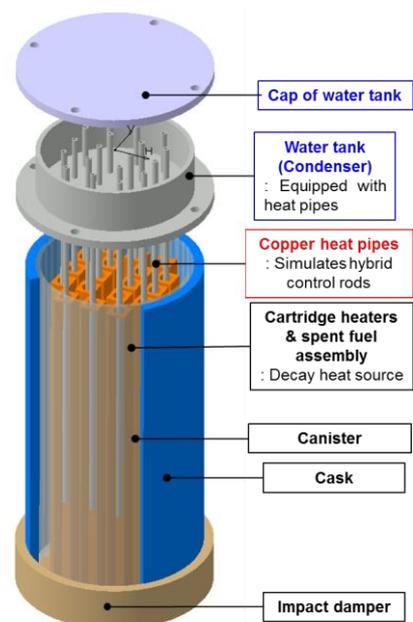
Fig. 1. Schematic of UCAN mock-up.
