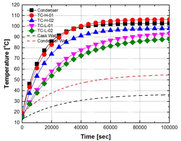
Fig. 3. Temperature evolutions of heat pipe-equipped canister with air condenser.
