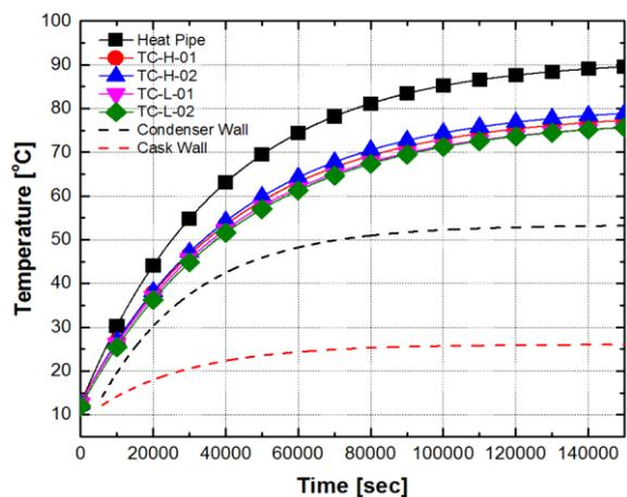
Fig. 4. Temperature evolutions of UCAN comprises water condenser and heat pipe.
