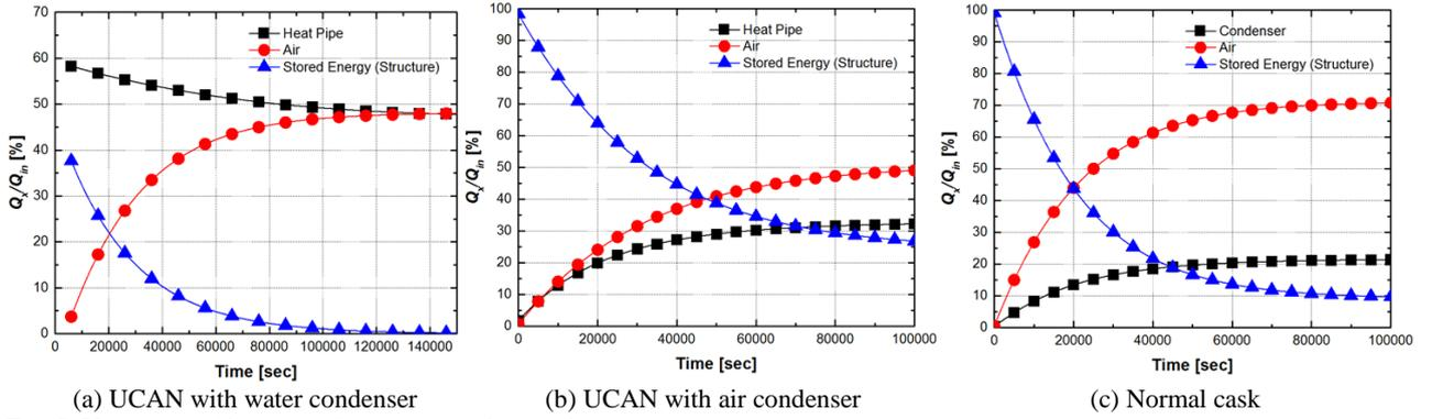
Fig. 5. Variations of heat transfer rates according to design of canisters.
