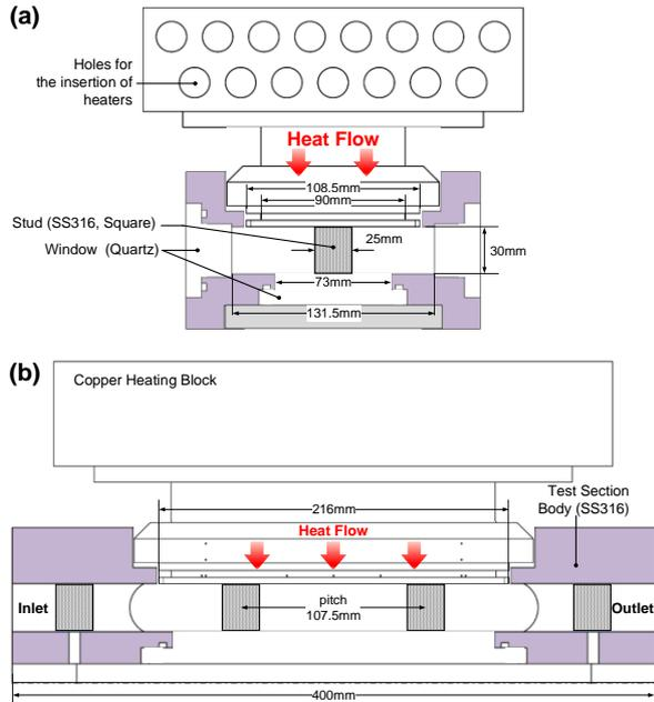
Fig. 2. Sectional views of test section with the aligned obstacles (stud); (a) transversal, (b) Longitudinal
