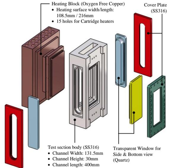
Fig. 1. Illustration of the test section assembly
