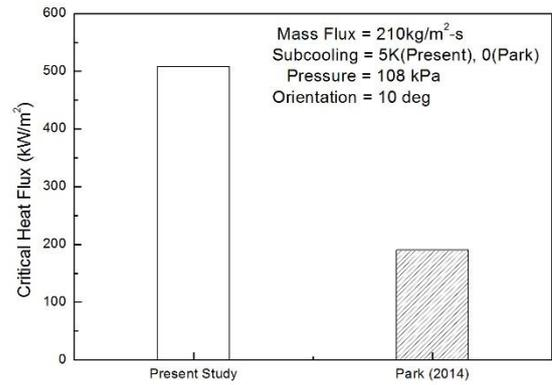
Fig. 3. Comparison of measured CHF with the model developed by Park (2014) under flow boiling
