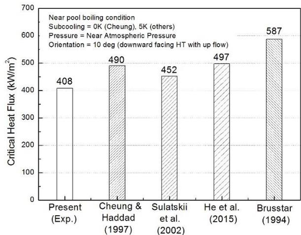
Fig. 4. Comparison of measured CHF with the models under pool boiling condition
