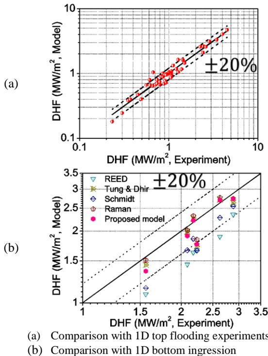
Fig. 4. Comparison with DHF experiments (with 20% of error lines)
