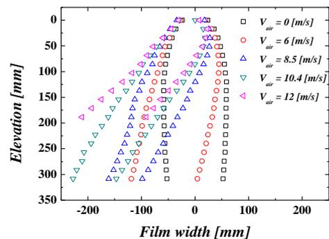
Fig. 2 Film width for 1/20 scale (water velocity :0.45m/s, air velocity:0, 6, 8.5, 10.4, 12m/s)
