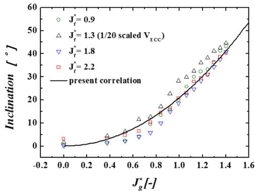
Fig. 3 Liquid film flow shift due to gas flow
