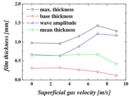
Fig. 3 Maximum film thickness, base film thickness, wave amplitude and mean film thickness when the liquid nozzle velocity is 0.45 m/s and the lateral gas velocity is 0 m/s, 3 m/s, 5 m/s, 7 m/s and 9 m/s.
