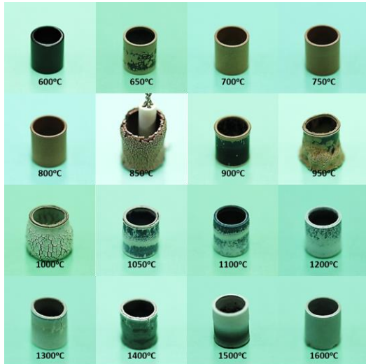
Fig. 1 Macro samples of air oxidized zircaloy-4
