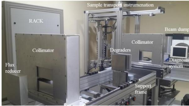
Fig. 2. The installed instrumentation for beam control and automatic sample transport and diagnosis system in target room.
