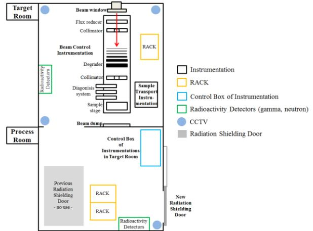
Fig. 1. The schematic of target and process rooms of 100-MeV low-flux proton beam facility.
