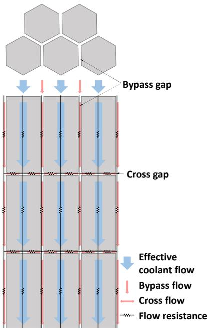
Fig. 1. Conceptual diagram of PMR core and flow network
