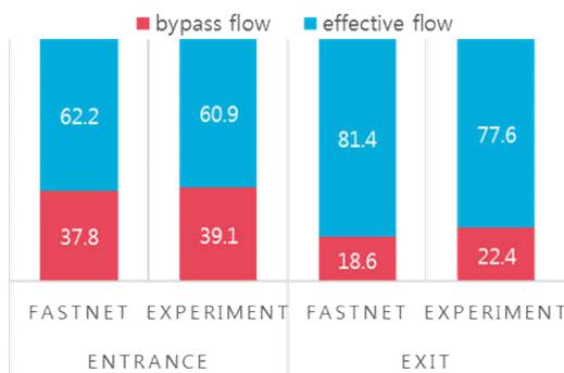
Fig. 6. Comparison results between experiment and FastNet: bypass flow ratio (BG6242-CG2)
