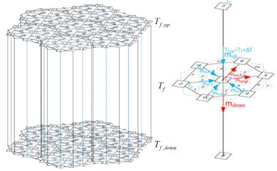
Fig. 3. Domain for fluid heat transfer analysis; temperature rising due to solid and lateral thermal fluid mixing
