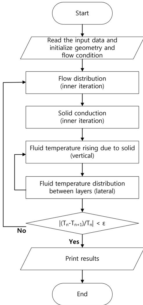
Fig. 5. Flow chart of FastNet calculation procedure
