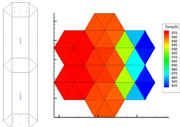
Fig. 8. FastNet single fuel assembly analysis and heat transfer analysis
