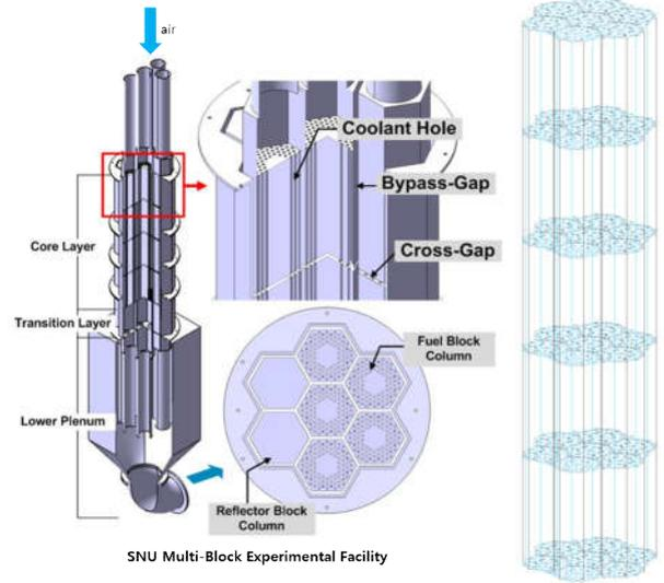
Fig. 4. SNU multi-block experimental facility [2] and 3-D flow network model for FastNet.
