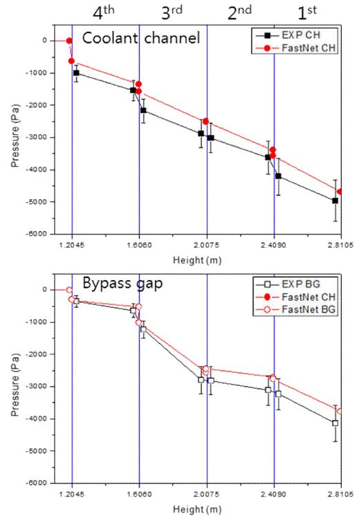
Fig. 7. Comparison results between experiment and FastNet: pressure drop (BG6242-CG2)
