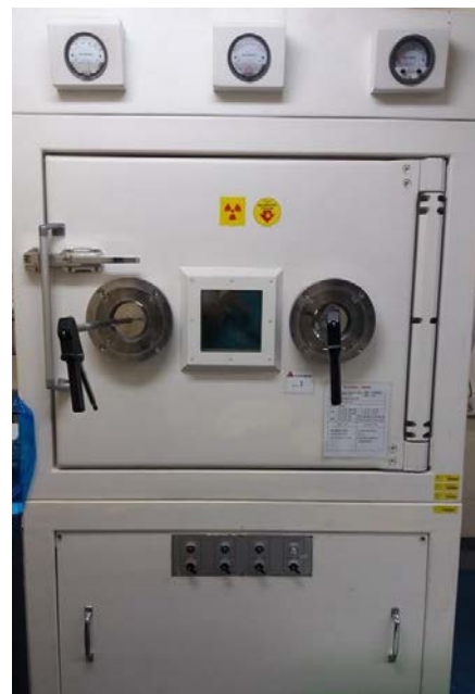
Fig. 1. A radiation-shielded micro-XRD system.
