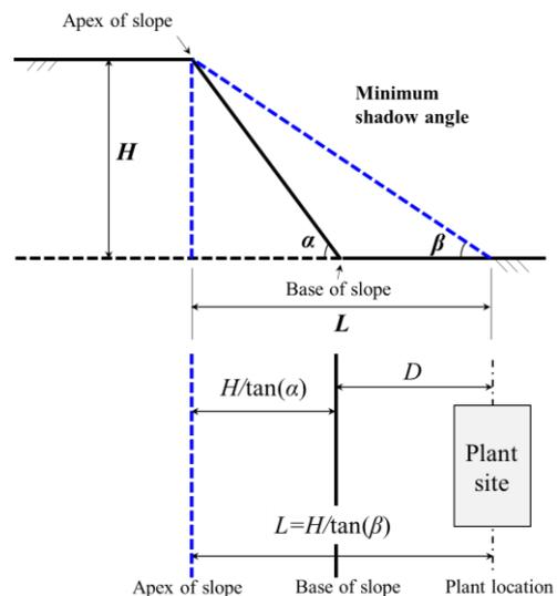
Fig. 2. Geometrical relation between slope and plant site
