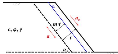
Fig. 1. Sliding block model used for seismic slope fragility analysis
