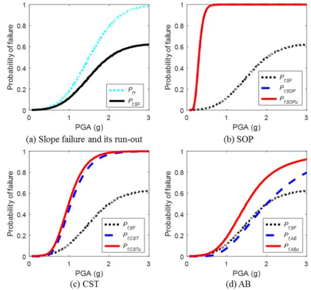
Fig. 4. Degraded fragility curves for SOP, CST and AB considering slope vulnerability causing a potential damage to NPP
