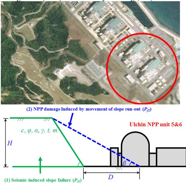
Fig. 3. Site of Ulchin NPP 5 & 6 and adjacent slope
