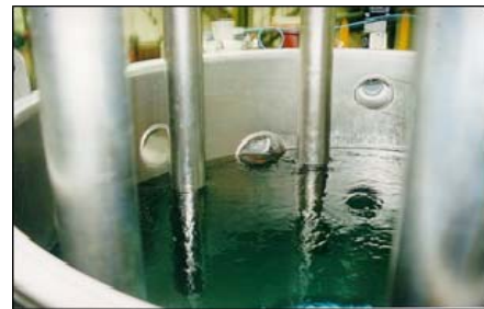
Fig. 1. Chemical decontamination (Medoc process at (BR3)
