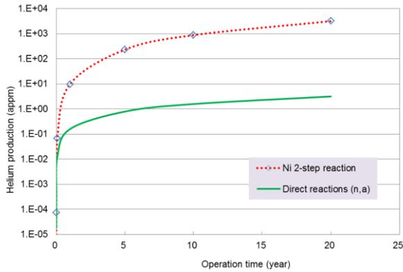
Fig. 3. Calculated He production for Inconel X-750 (1 gram) in the spacer of CANDU reactor
