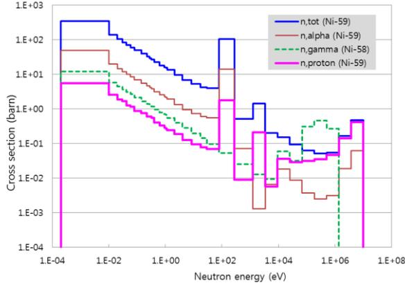
Fig. 2. Neutron reaction cross sections for  $^{59}\text{Ni}$  total,  $^{59}\text{Ni}(n,\alpha)$ ,  $^{58}\text{Ni}(n,\gamma)$  and  $^{59}\text{Ni}(n,p)$  reactions as a function of neutron energy
