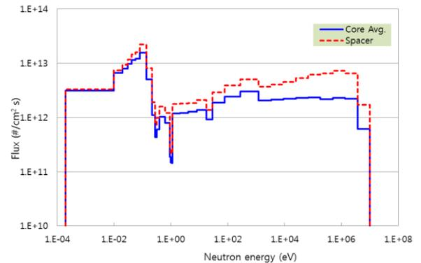
Fig. 1. Neutron spectra for an average CANDU channel power and X-750 spacer
