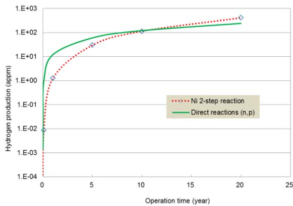
Fig. 4. Calculated H production for Inconel X-750 (1 gram) in the spacer of CANDU reactor
