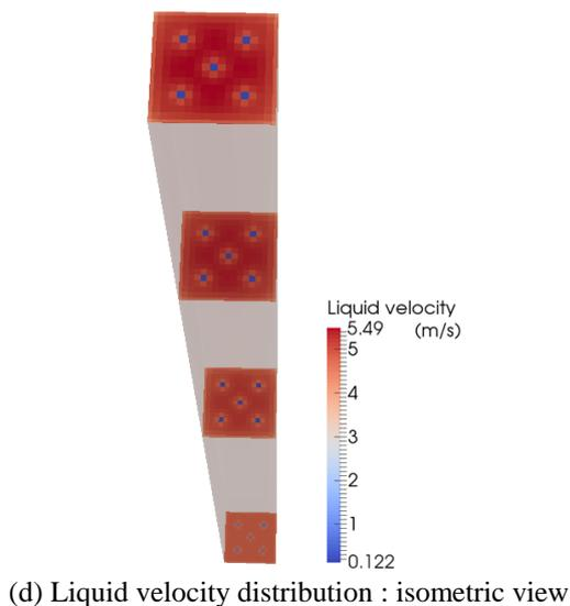
**Fig. 5. Imposed power, calculated temperature and calculated liquid velocity distribution**
