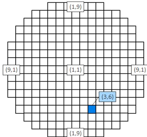
Fig. 4. Location of the imposed power distribution of the calculation of single assembly
