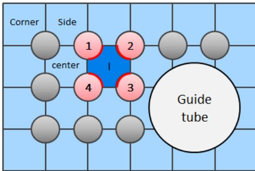
Fig. 2. Schematic view of subchannels
