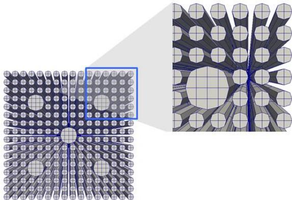
Fig. 3. Modeling of 16x16 single assembly including guide tube model
