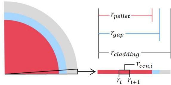
Fig. 1. Schematic view of one-dimensional heat transfer inside of the fuel rod
