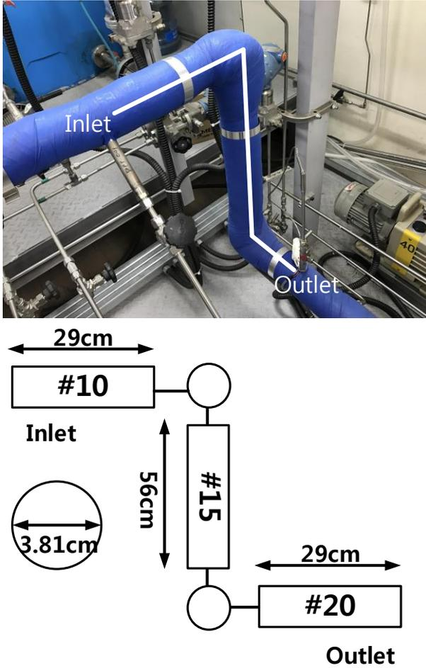
Fig. 3. The overall view and schematic diagram of the test section for the pressure drop test
