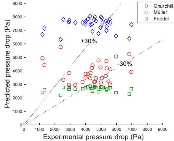
Fig. 5. The comparison results of the measured and predicted pressure drop according to the pressure drop correlations
