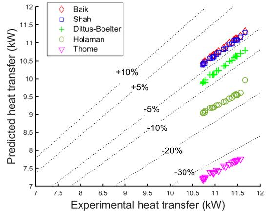
Fig. 4. The comparison results of the measured and predicted heat transfer according to the heat transfer correlations
