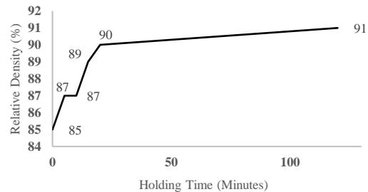
Fig.4-C. Effect of holding time on density under constant temperature and pressure conditions
