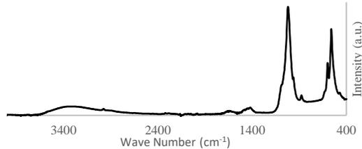
Fig. 2. FTIR spectra of the synthesized hydroxyapatite.
