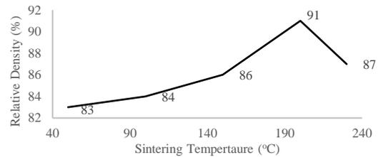
Fig.4-A. Effect of sintering temperature on density.
