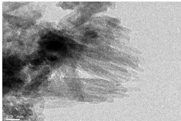
Fig.3. TEM image of the hydroxyapatite powder showing the nano rod like morphology of the synthesized powder.
