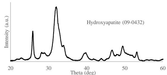
Fig. 1. XRD patterns of the synthesized dried calcium hydroxyapatite showing no other phase except apatite.
