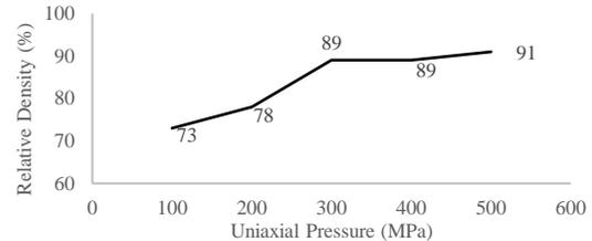
Fig.4-B. Effect of applied pressure on the density under constant temperature conditions.
