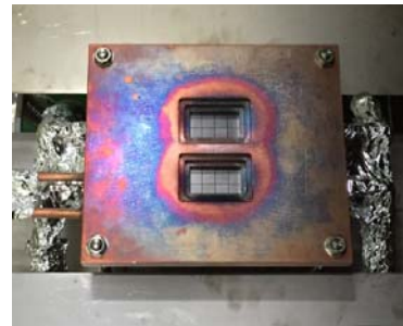
Fig. 3. Target assembly of W/Cu bonding mockups for KSTAR
