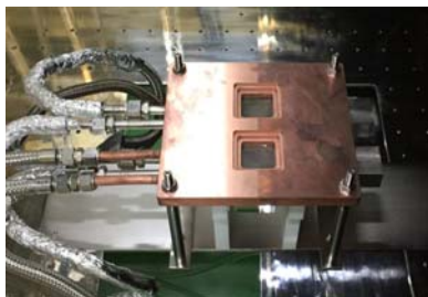
Fig. 1. Target assembly of W/FMS (Grade.91) bonding mockups by using HIP technology
