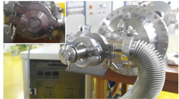
Figure 4. Vacuum stability test of the exit window using havar foil.
