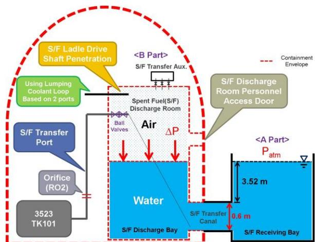
Fig. 1. Schematic diagram of leakage paths of S/F discharge room during S/F transfer
