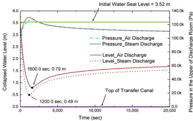
Fig. 4. Water level behavior of S/F discharge room
