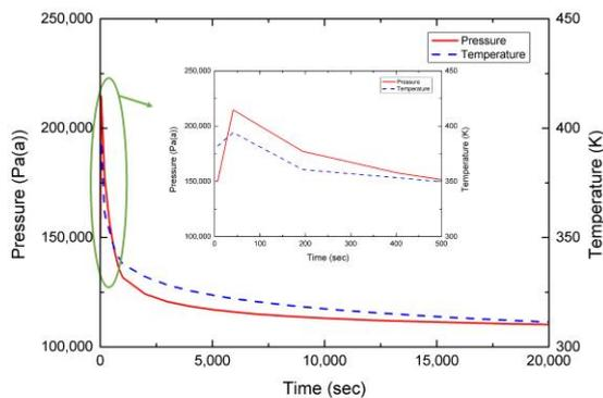
Fig. 2. The pressure and temperature conditions of the containment in the event of a LOCA with the total loss of dousing spray (100% ROH).
