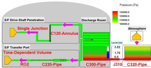
Fig. 5. Results of analysis in the case of air discharge after the peak of the induced pressure
