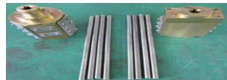
Fig. 2. Blade types and simulated fuel rods. (2-CUT module and 3-CUT module)
