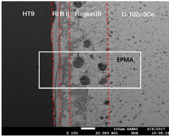
Fig. 3. Cross sectional SEM image at the interface between U-10Zr-5Ce and HT9
