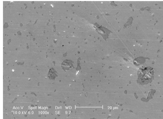
Fig. 2. SEM image of as-injection casted U-10Zr-5Ce
