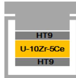
Fig. 1. Schematic diagram of the holder
