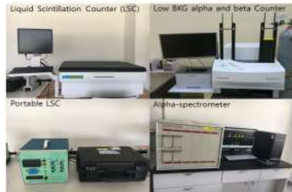
Figure 2. Analysis equipment installed currently for the environmental sample analysis system
