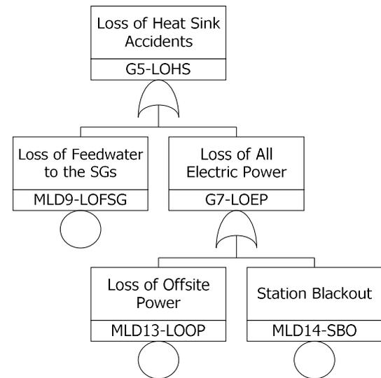
Fig. 6. The Master Logic Diagram (MLD) of PGSFR (5/6).
