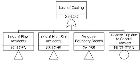
Fig. 4. The Master Logic Diagram (MLD) of PGSFR (3/6).
