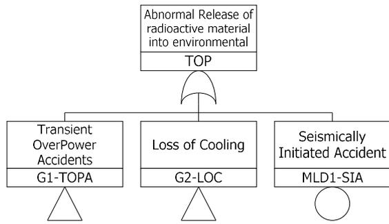
Fig. 2. The Master Logic Diagram (MLD) of PGSFR (1/6).
