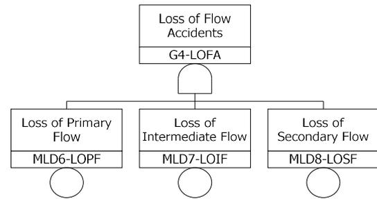
Fig. 5. The Master Logic Diagram (MLD) of PGSFR (4/6).
