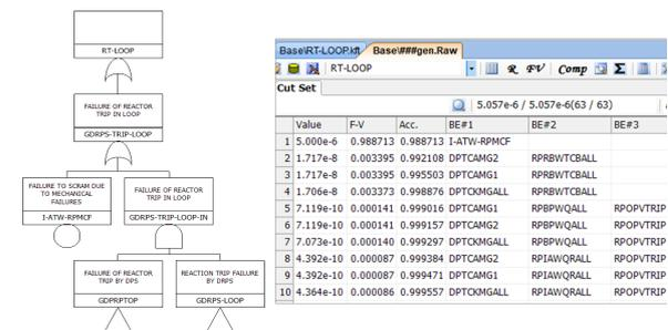
Fig. 9. The fault tree and calculated failure probability for RT.
