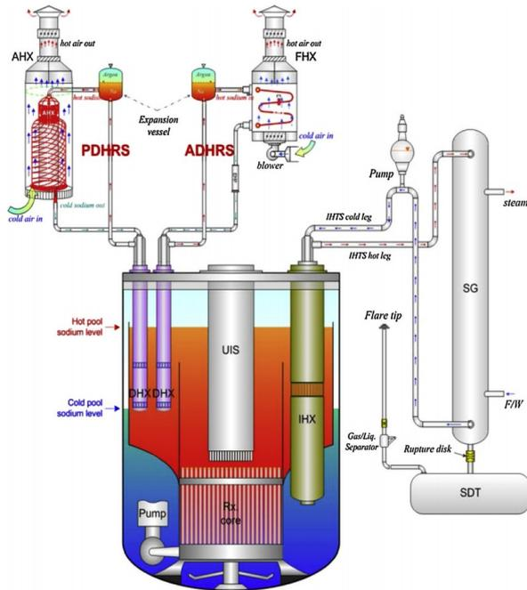
Fig. 1. The conceptual design of PGSFR [5].
