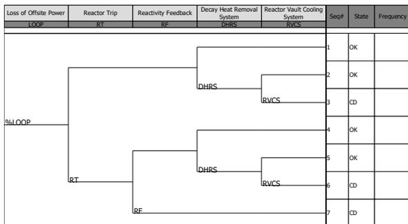
Fig. 8. The loss of offsite power (LOOP) event tree.
