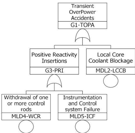
Fig. 3. The Master Logic Diagram (MLD) of PGSFR (2/6).
