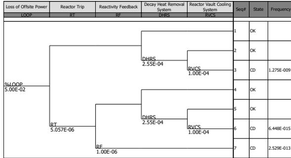
Fig. 10. The accident sequences quantification result for LOOP.
