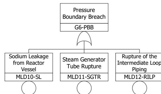
Fig. 7. The Master Logic Diagram (MLD) of PGSFR (6/6).
