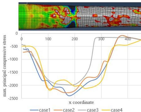
Fig. 4. Maximum principal compressive stress of Zircaloy-4 tube at case1-4
