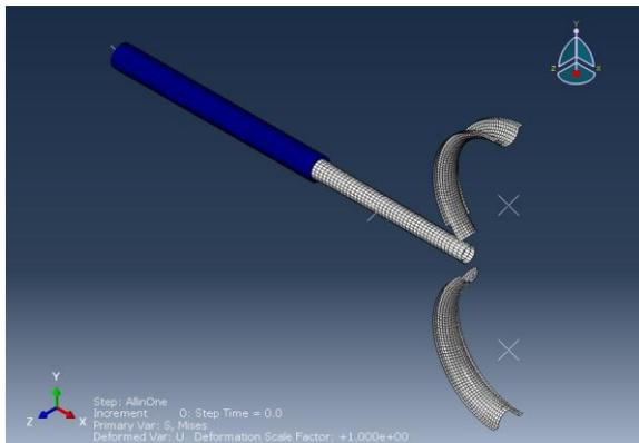
Fig. 3. Pilgering simulation model
