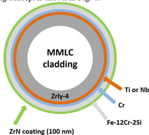
Fig. 1. Description of MMLC cladding cross-section
