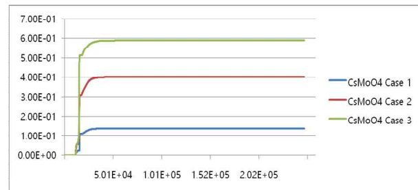
Fig. 5. CsMoO 4 release fraction according to break position
