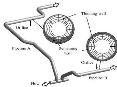
Fig. 1. Schematic layout of pipeline in Mihama PWRs [3].
