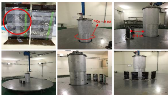
Fig. 1. Experimental of gamma-ray irradiation in NPT-IGBT
