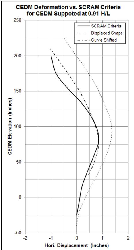
Fig. 5 Comparison of CEDM Deformation and Scram Criteria
