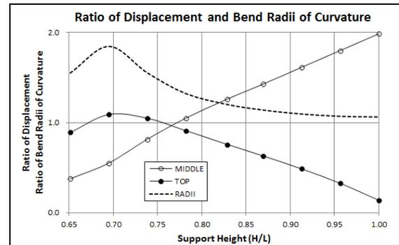
Fig. 4 Ratio of Displacement and Bend Radii of Curvature
