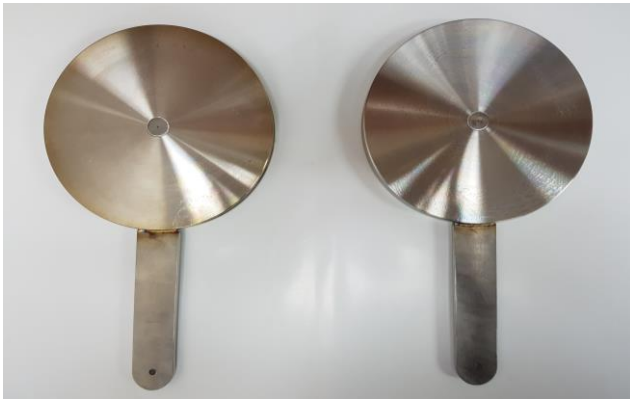
Fig. 4. Feature of nozzle (with the diameter of 1.5 mm and length of 5.0 mm)
