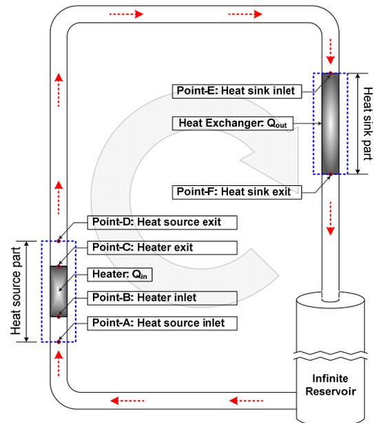
Fig. 1 Schematic of the postulated closed loop system for numerical investigation
