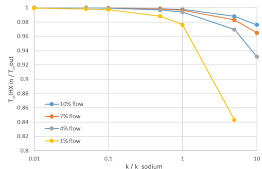
Fig.4 Variation of temperature ratios at the heat sink inlet (point-E) to the heat source exit (point-D)
