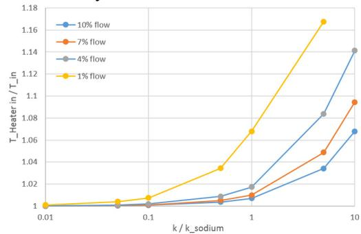
Fig.3 Variation of temperature ratios at the heater inlet (point-B) to the heater source part (point-A, ideal)
