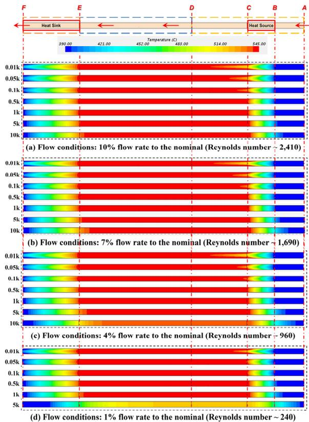
Fig.2 Temperature distribution along the flow direction in the test loop configuration
