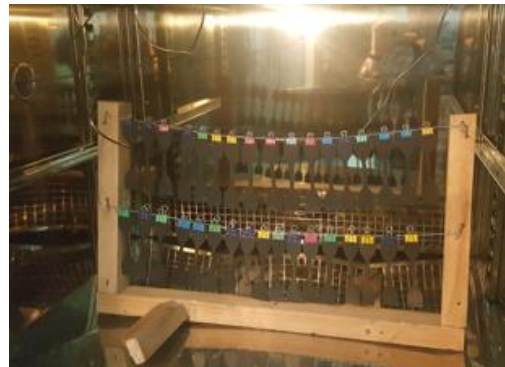
Fig. 1. Accelerated thermal aging test
