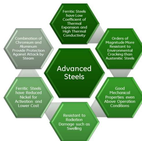
Figure 1: Desirable characteristics of ferritic steels for ATF cladding [5]
