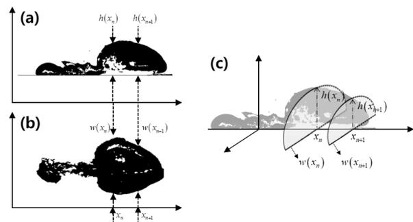
Fig. 2. Image reduction process; by coupling (a) side view image and (b) top view image, volume of slug was measured by integration according to each times
