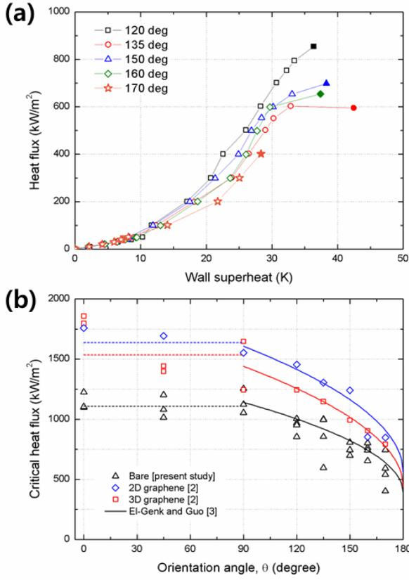
Fig. 3. (a) Boiling curve, and (b) CHF vs orientation
