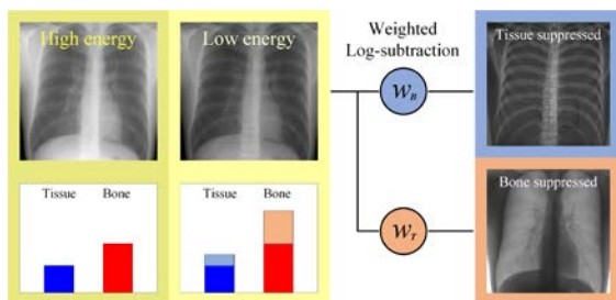
Fig. 1. Concept of weighted log-subtraction for dual-energy imaging.
