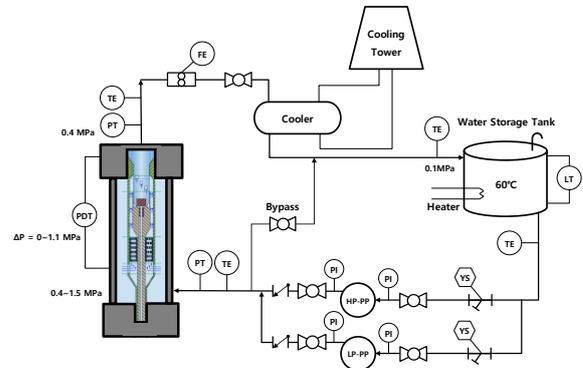
Fig. 3. Conceptual design of the test loop facility.
