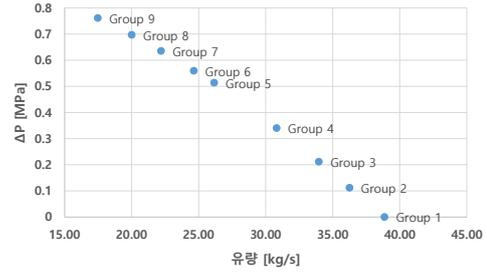
Fig. 2. Estimated flow rates and pressure drops across the core receptacle model for the performance test.
