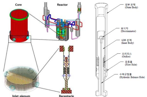
Fig. 1. Location and internal structures of the receptacle.
