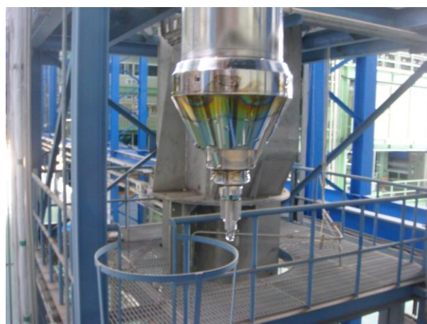
Fig. 4. New designed capsule after out-pile testing for 15 cycles (450 days)
