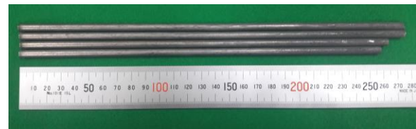
Fig. 2. Re-fabricated U-10wt%Zr-5wt%RE metallic fuel slugs
