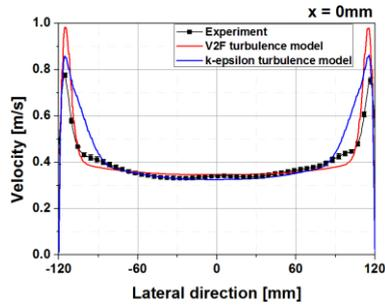
Fig. 9. Vertical velocity profiles from the experiment and CFD analysis at the mid-plane
