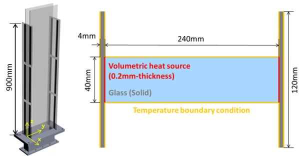
Fig. 2. The design of the test section (left) and the top view of calculation geometry for CFD analysis (right)
