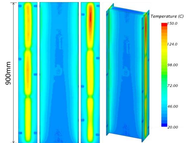
Fig. 3. Measured outer wall temperature distributions (left) and temperature boundary conditions imposed on the calculation geometry of the CFD analysis (right)
