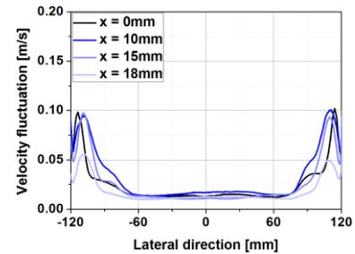
Fig. 8. Fluctuation profiles of the vertical velocity components at  $z = 0.8$  m and at  $x = 0$  mm,  $10$  mm,  $15$  mm and  $18$  mm
