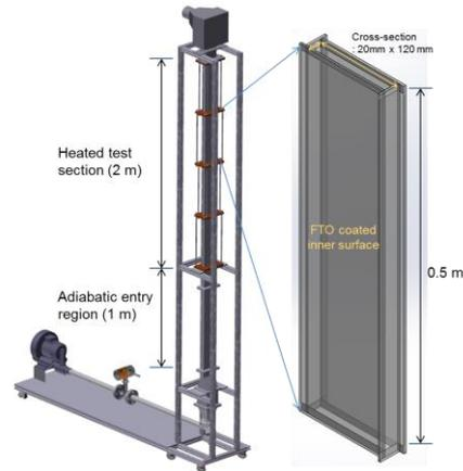
Fig. 11. Schematics of the newly designed experiment facility (left) and its design of the heated test section (right)
