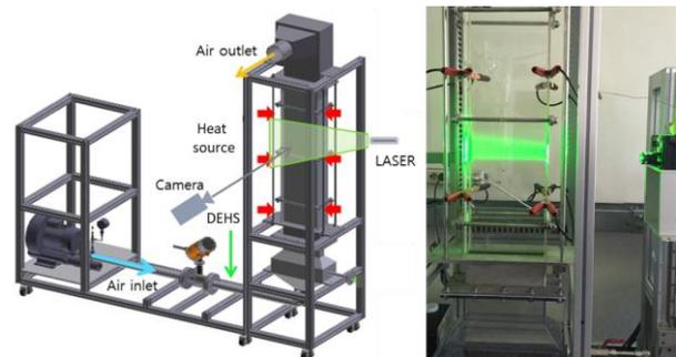
Fig. 1. The design of the flow visualization test facility (left) and the picture of its test section (right) [8]
