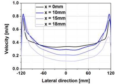
Fig. 6. Vertical component velocity profiles at  $z = 0.8$  m and at  $x = 0$  mm,  $10$  mm,  $15$  mm and  $18$  mm from the mid-plane
