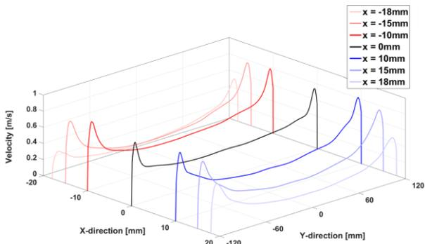
Fig. 5. Vertical velocity components of the obtained local flow structure at  $z = 0.8$  m from the entrance of the test section at the 7 different positions in the depth direction
