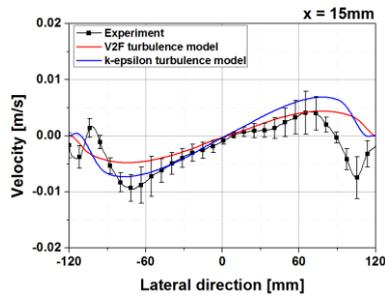
Fig. 10. Horizontal velocity profiles from the experiment and CFD analysis at  $x = 15\text{mm}$  from the mid-plane
