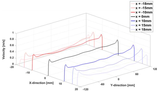
Fig. 4. Vertical velocity components of the obtained local flow structure at  $z = 0.2$  m from the entrance of the test section at the 7 different positions in the depth direction
